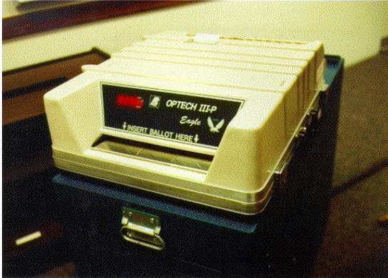
**Figure 1: A Precinct-based optical scan system (the ES&S Optech Eagle)**
